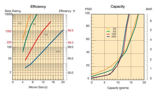
Results typical from Multi-pass tests run per test standard ISO 16889 @ 15 gpm to 100 psid terminal - 10 mg/L BUGL Refer to Appendix for relationship to test standard ISO 4572.
