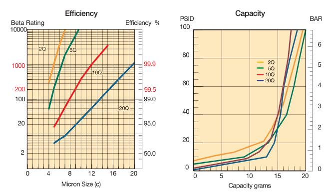
Results typical from Multi-pass tests run per test standard ISO 16889 @ 20 gpm to 100 psid terminal - 10 mg/L BUGL Refer to Appendix for relationship to test standard ISO 4572.
