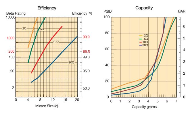
Results typical from Multi-pass tests run per test standard ISO 16889 @ 10 gpm to 100 psid terminal - 10 mg/L BUGL Refer to Appendix for relationship to test standard ISO 4572.
