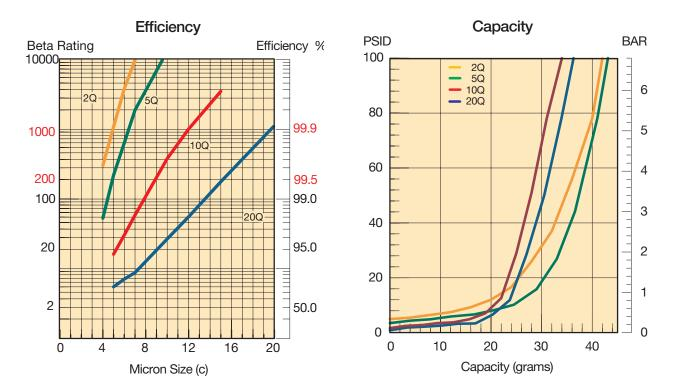
Results typical from Multi-pass tests run per test standard ISO 16889 @ 30 gpm to 100 psid terminal - 10 mg/L BUGL Refer to Appendix for relationship to test standard ISO 4572.
